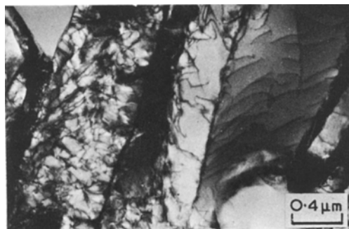
Figure 1 Single phase dislocated lath martensite structure of the beta quenched alloys.
